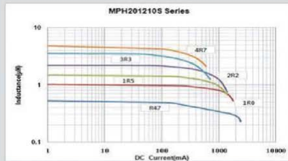
Inductance vs. DC Current Characteristics
