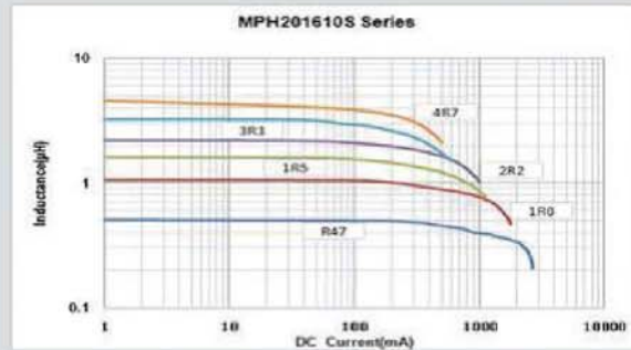
Inductance vs. DC Current Characteristics
