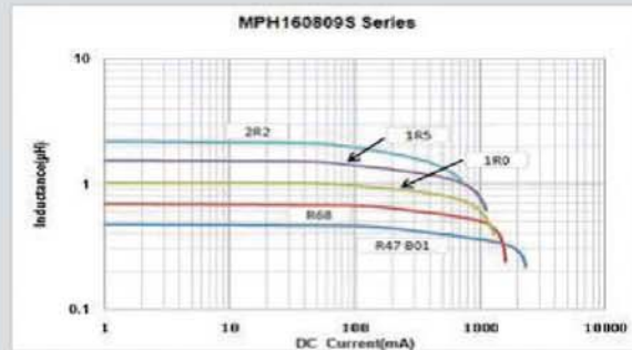
Inductance vs. DC Current Characteristics
